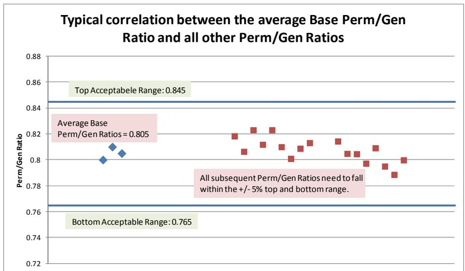
**Figure 3–5.** Typical Correlation between the averaged Base Perm/Gen Ratio and Subsequent Perm/Gen Ratios
