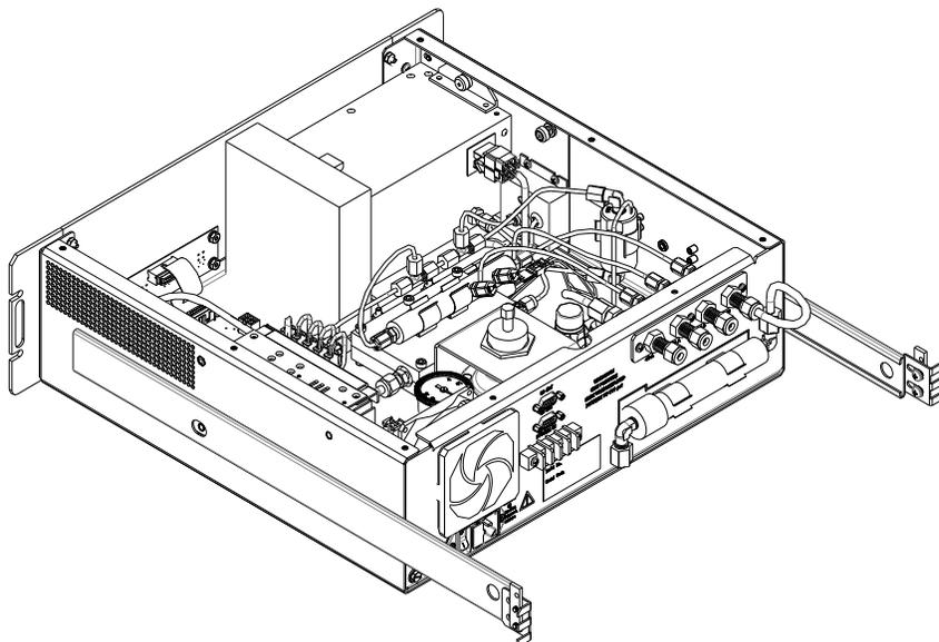
**Figure 4–5.** Replacing the Pressure Transducer Assembly
