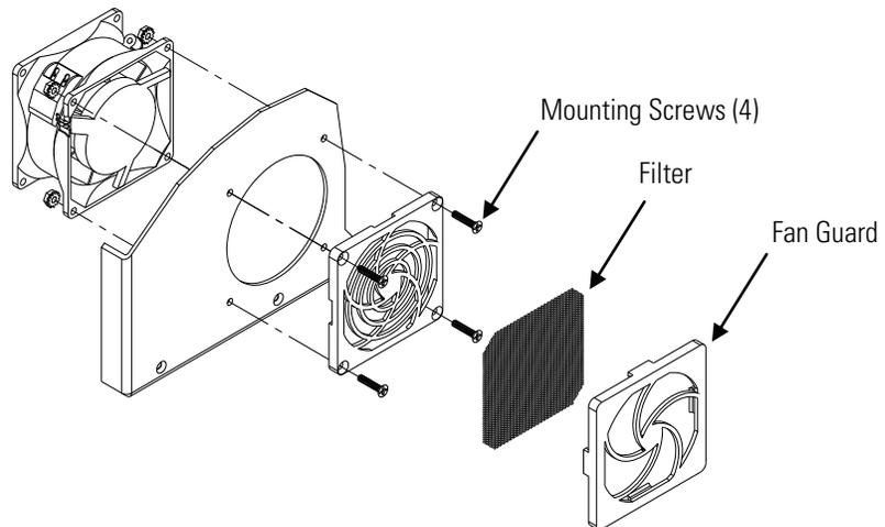
**Figure 4-1.** Replacing the Fan
