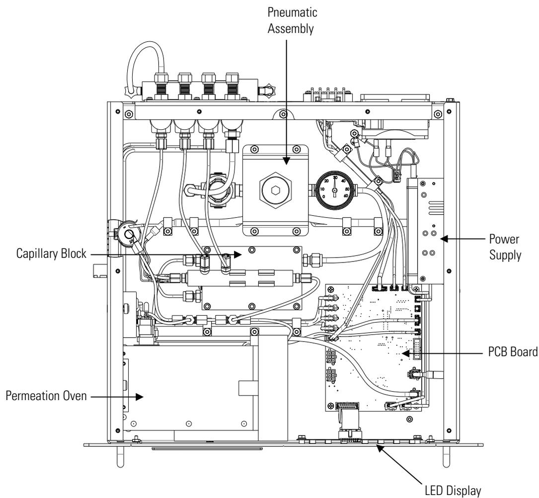
**Figure 1–2.** Model 84*i* Component Layout
