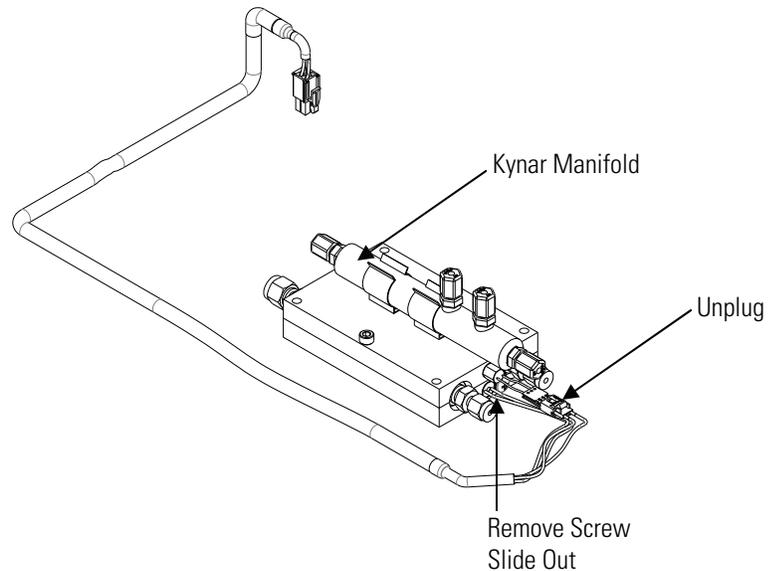
**Figure 4-6.** Flow Splitter Assembly
