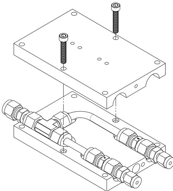
**Figure 1–4.** Capillary Block Assembly
