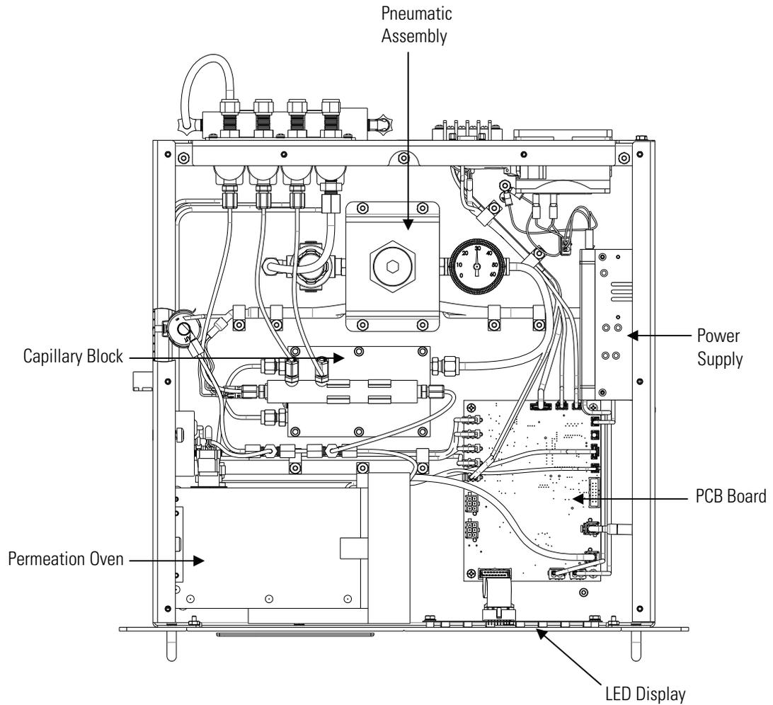
**Figure 4–9.** Model 84*i* Component Layout
