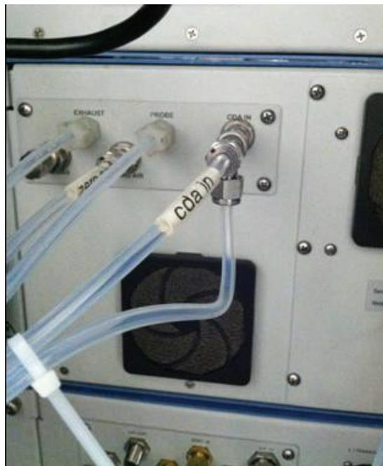
**Figure 2–6.** Retrofitted 81*i* CDA Plumbing to Support 84*i*
