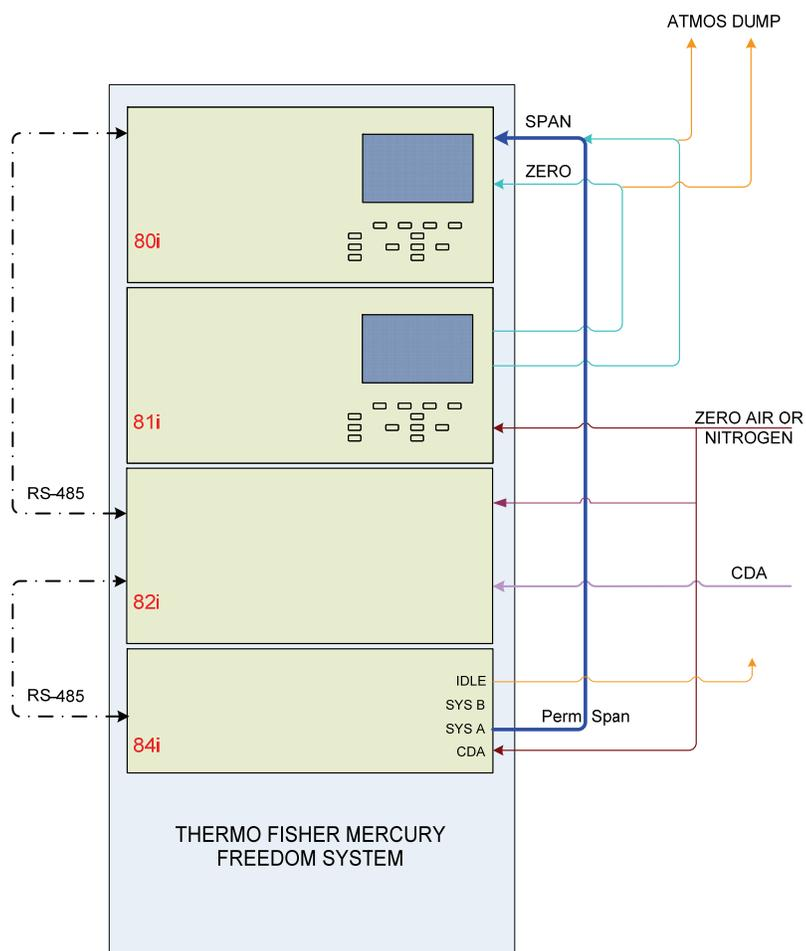
**Figure 3–1.** Tubing and Electrical Configuration
