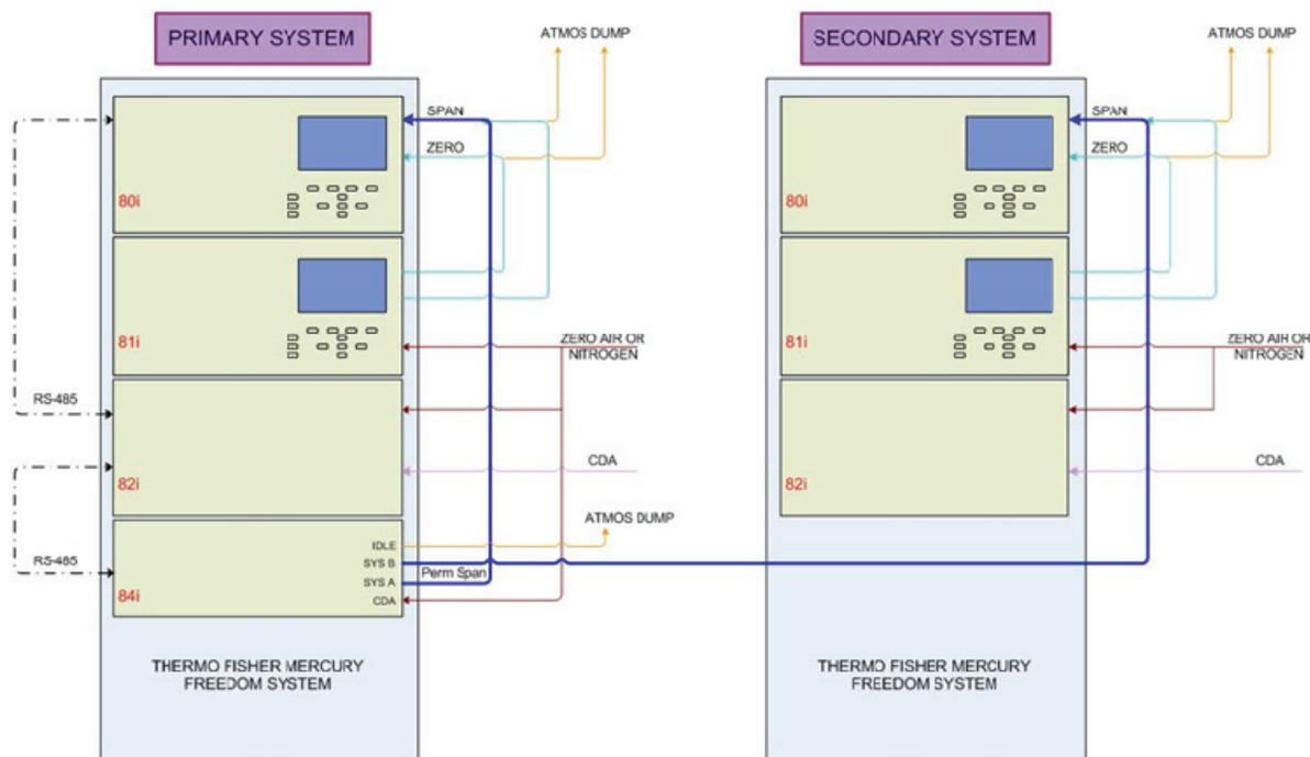
**Figure 3–3.** Physical and Electrical Connections for auditing two Mercury Freedom Systems using one 84i Permeation Source
