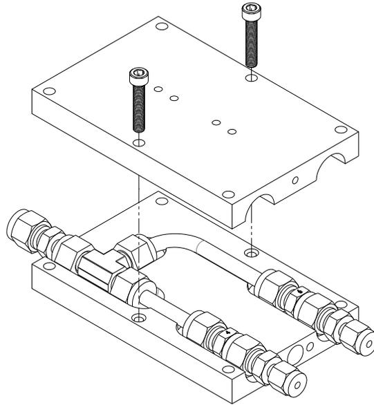
**Figure 4–7.** Capillary Block Assembly
